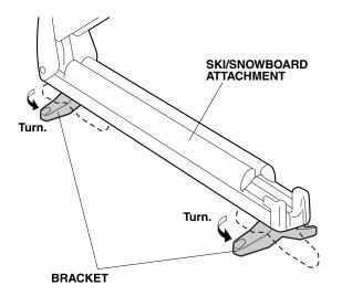
4. Using the wrench supplied, install the ski/snowboard attachment to the front crossbar with four bolts, four collars, and two brackets.
