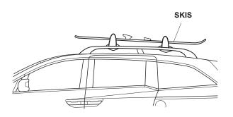
9. If the bindings cannot be positioned between the front and the rear attachments, install the skis with the rear bindings behind the rear attachment as shown.
